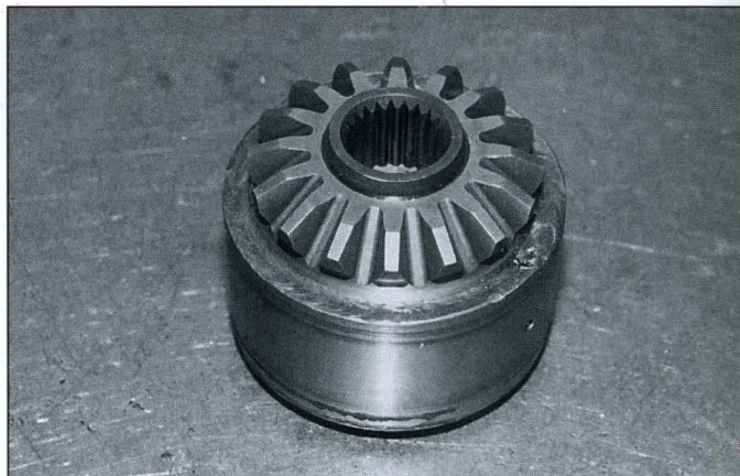
Right side of coupling unit has new side gear welded to it.
