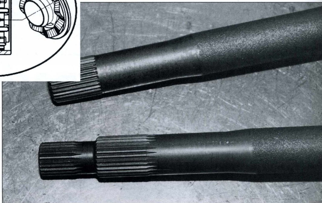
Axles must be replaced – now you can see why left-hand axle has special spline extension which fits into coupling unit.
