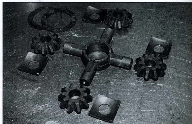
Four pinion gears are used to reduce stress and increase power capacities.
