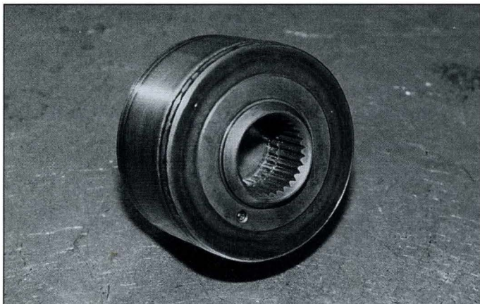
Left side of coupling unit accepts specially splined axle.
