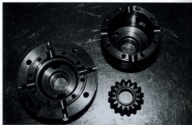
Hydratrak carrier assembly replaces factory unit.
